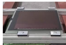
Test assembly for hail impact test
