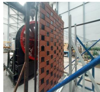
Set-up for dynamic wind load test as part of ageing sequence
