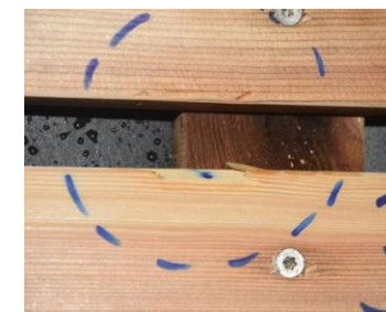
Minor dent and edge chipping at the point of impact of the ice ball.
