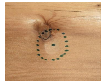
Minor dent and discoloration at the point of impact of the steel ball.
