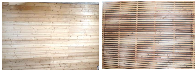
Tested specimens: Tongue and Groove Boards (left) and Wooden Slats with Dilatation (right) by RIKO Hiše
