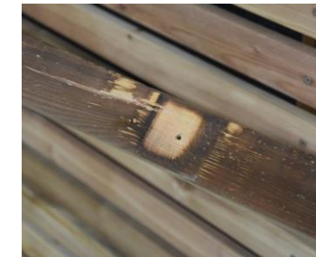
Minor discolorations and chipping after artificial ageing.
