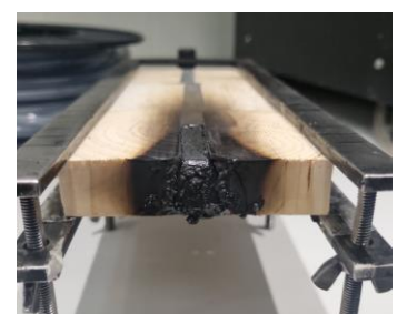
Small flame edge exposure for 30 s results in ignition of the flexible joint and dropping of flaming material.
