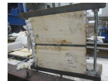
Flexible joint in tension after fire resistance test: unexposed side (left), exposed side (right).
