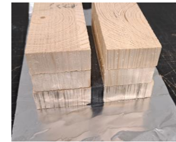
Cone calorimeter test of flexible joint – simulation of reduction of material.
