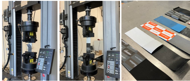
Preparation and testing of tape-membrane joints at M&S Lab
